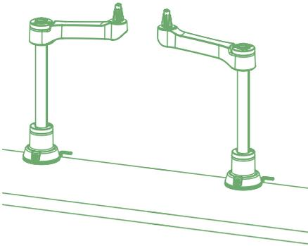
Rotate the arm, and check whether it stops at the chosen side. If not, take the forearm off the pole, and place it exactly opposite on the pole. Rotate it again to check if it stops at the desired side. Rotate the forearm in the right position in such way that the arm cannot move backwards but only forward.
